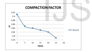
The table indicates that the compacting factor values get reduced on increasing the RHA content. The compacting factor values reduced from 0.91 to 0.79 as the percentage RHA replacement increased from 0% to 25%. These results indicate that the concrete becomes less workable asthe RHA percentage increases meaning that more water is required to make the mixes more workable. The high demand for water as the RHA content increases is due to increased amount of silica in the mixture.
